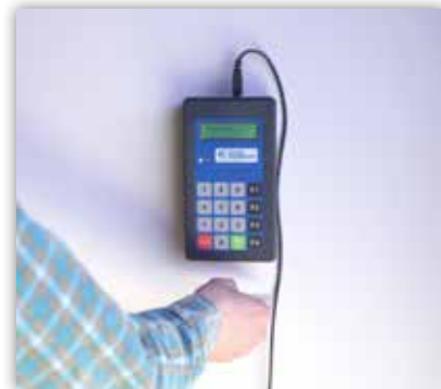
Self-service keypad/scanner directly connected to network *Printer not supported
